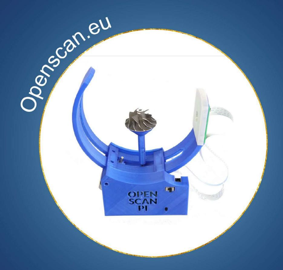
Based on Photogrammetry, the OpenScan 3D Scanner is compatible with a variety of cameras, thus enabling use with simple smartphones or DSLR. In order to create a 3D model, the device captures pictures from various views and using Freeware, creates a highly accurate 3D model with or without texture.
