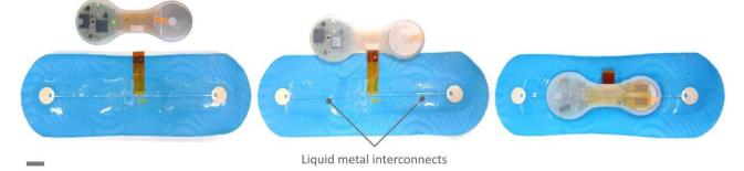
Figure 1 - Photographs of the wireless wearable device consisting of the electronic module and the soft and stretchable sensor patch with patterned liquid metal interconnects for electrophysiological readouts. The scale bar corresponds to 1 cm.
