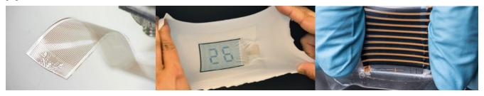
Devices from left to right: stretchable high resolution neural electrode, printed stretchable display, stretchable thermoelectric generator.
