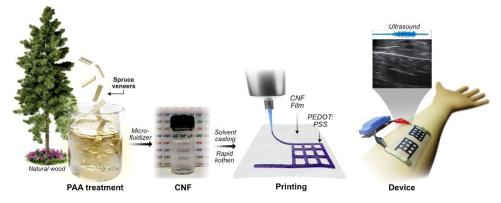
Figure 1. Schematic of CNF prepared from wood, conductive polymers printed on the surface of CNF film, and signals collecting of musculoskeletal tissue.
