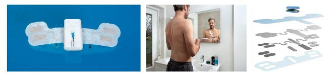
Figure 2. The Nighthawk health patch platform with dry adhesive electrodes for continuous and remote monitoring of ECG and bio-impedance during multiday wear time.
